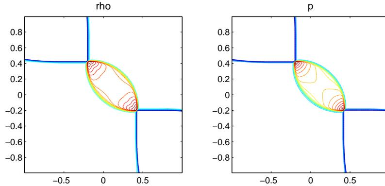
Figure 5: Two dimensional Riemann problem with four shocks. Isolines of density and pressure calculated on a  $400 \times 400$  mesh at time  $T = 0.25$
