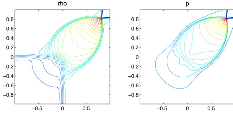
Figure 4: Two dimensional Riemann problem containing two shocks/two slip lines. Isolines of density and pressure calculated on a  $400 \times 400$  mesh at time  $T = 0.52$
