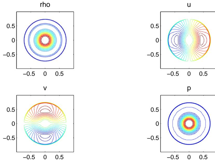
Figure 3: Cylindrical explosion problem: Isolines of the solution calculated on a  $400 \times 400$  mesh at time  $T = 0.2$
