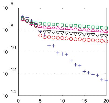
**Figure 4.** Singular values of the measurement operators  $G_{\delta,n}^h$  (+ without additional noise,  $\circ$  with 3% noise,  $\nabla$  with 10% noise,  $\triangle$  with 25% noise,  $\square$  with 50% noise).
